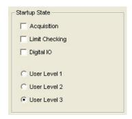
Used to set the default startup state for the project's **Acquisition**, **Limit Checking**, and **Digital IO** processes. eZ-TOMAS will turn on the selected processes when the project is opened. The default user level (1, 2, or 3) is also selected in this panel.
