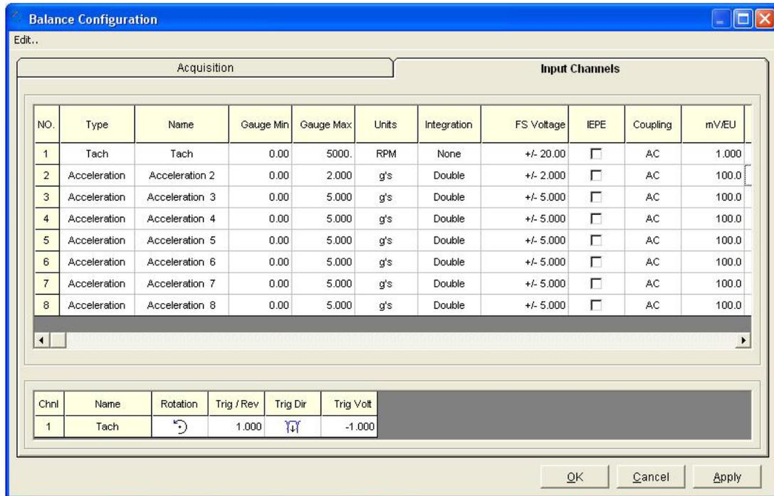
**Balance Configuration Input Channels Tab**
