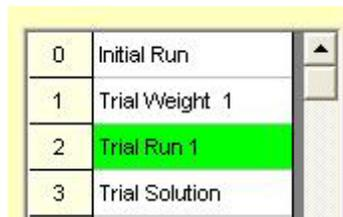
Use the same vibration acquisition method to obtain Trial Run Vibration data. Repeat these operations for each Balance Plane.
